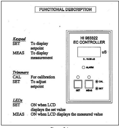
Figure 2.4 Conductivity Probe Display
